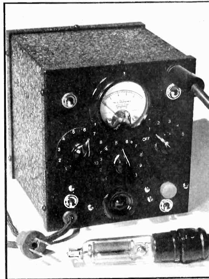
The timing-control-photometer-relay, mounted in a 6x6x6-inch cabinet. The phototube plugs in from a six-foot shielded cable
