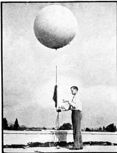
This Caltech explorer balloon travels 60,000 feet up with one pound of equipment, including a radio transmitter, an aneroid barometer, bimetallic thermometer, and humidometer. These instruments control clock-work contactors in the transmitter
